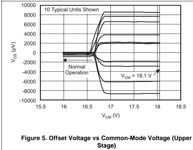
Figure 5. Offset Voltage vs Common-Mode Voltage (Upper Stage)
