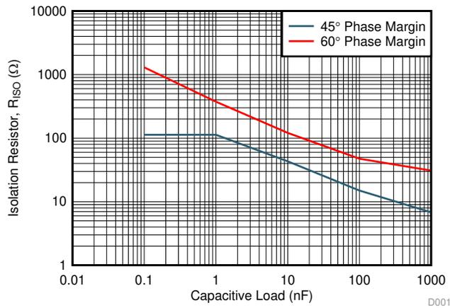
Figure 45. R<sub>ISO</sub> vs C<sub>LOAD</sub>
