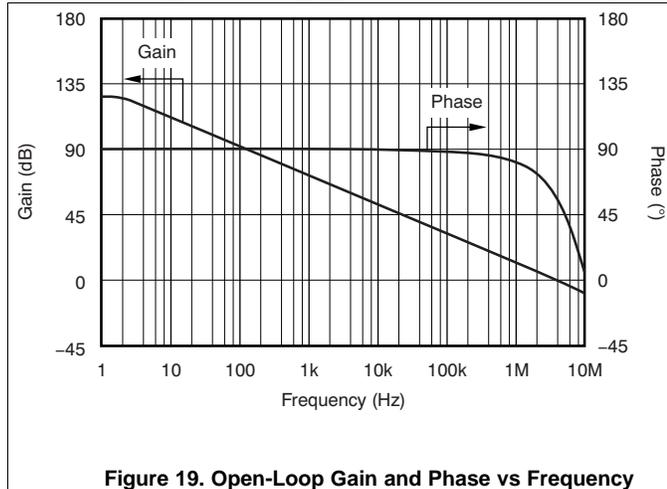
Figure 19. Open-Loop Gain and Phase vs Frequency
