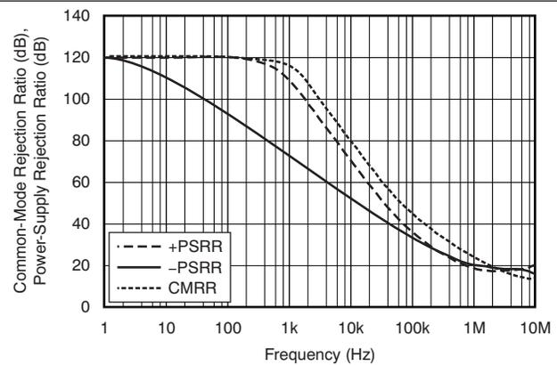
Figure 10. CMRR and PSRR vs Frequency (Referred-to Input)
