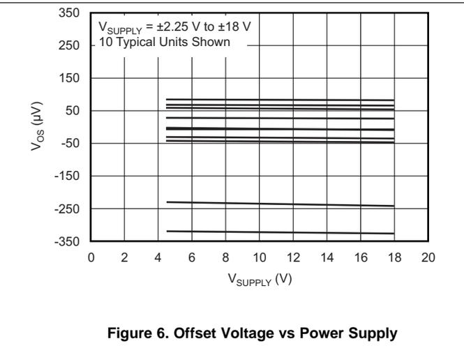
Figure 6. Offset Voltage vs Power Supply
