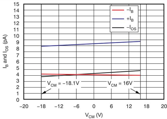
Figure 7.  $I_B$  and  $I_{OS}$  vs Common-Mode Voltage
