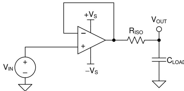
Figure 41. Unity-Gain Buffer With  $R_{ISO}$  Stability Compensation
