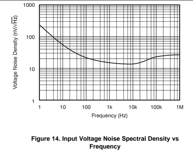
Figure 14. Input Voltage Noise Spectral Density vs Frequency
