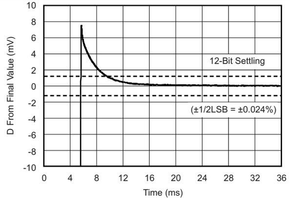
Figure 32. Large-Signal Settling Time (10-V Positive Step)
