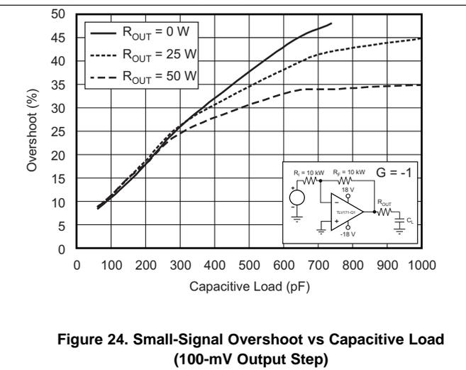
Figure 24. Small-Signal Overshoot vs Capacitive Load (100-mV Output Step)
