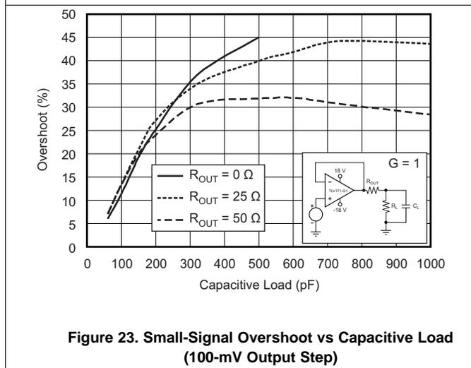
Figure 23. Small-Signal Overshoot vs Capacitive Load (100-mV Output Step)
