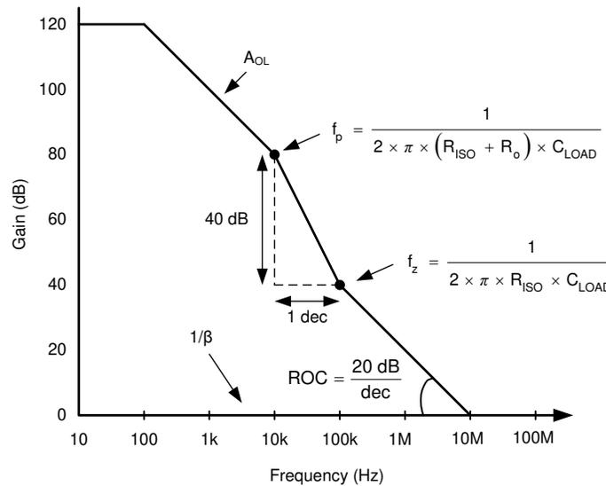
Figure 42. Unity-Gain Amplifier With R<sub>ISO</sub> Compensation
