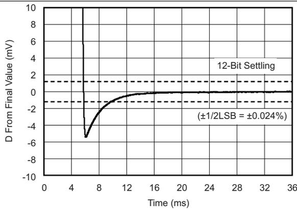
Figure 33. Large-Signal Settling Time (10-V Negative Step)
