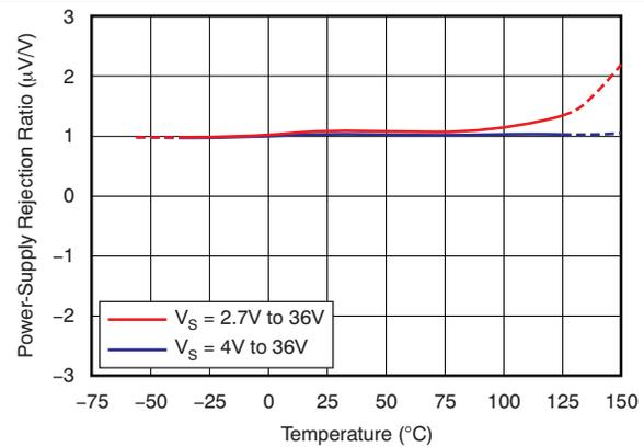
Figure 12. PSRR vs Temperature
