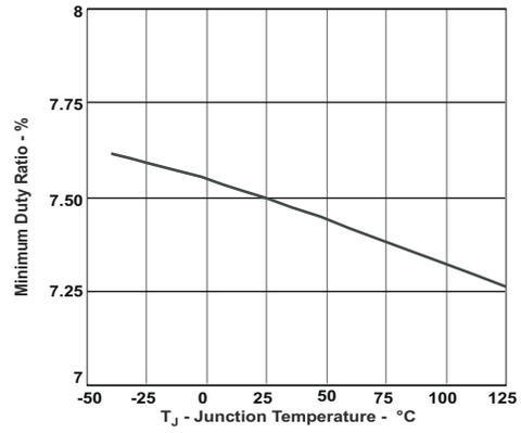
**Figure 5-8. Minimum Controllable Duty Ratio vs. Junction Temperature**
