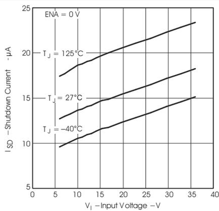
**Figure 5-3. Shutdown Quiescent Current vs. Input Voltage**
