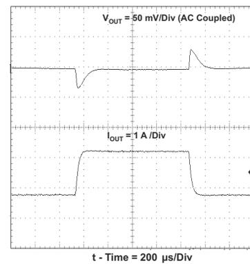
**Figure 7-7. Transient Response,  $I_O$  Step 0.75 to 2.25 A.**
