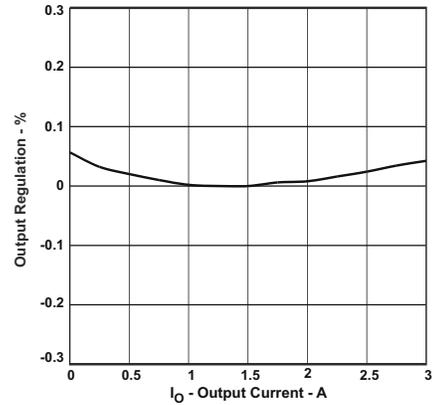
**Figure 7-3. Output Regulation % vs. Output Current**
