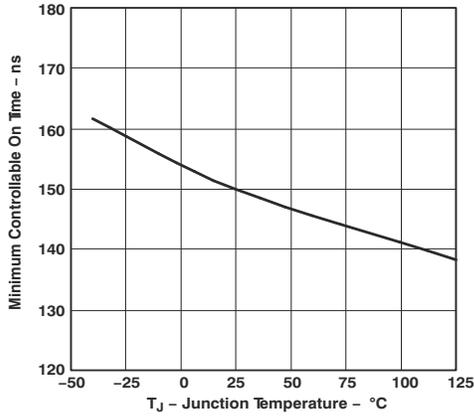
**Figure 5-7. Minimum Controllable On Time vs. Junction Temperature**
