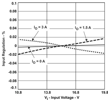
**Figure 7-4. Input Regulation % vs. Input Voltage**
