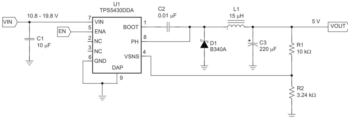
**Figure 7-1. Application Circuit, 12 V Input to 5.0 V Output**
