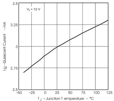
**Figure 5-2. Non-Switching Quiescent Current vs. Junction Temperature**
