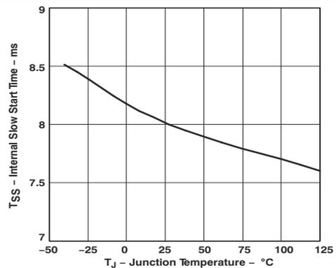
**Figure 5-6. Internal Slow Start Time vs. Junction Temperature**
