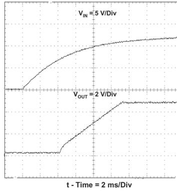
**Figure 7-8. Startup Waveform,  $V_{IN}$  and  $V_{OUT}$ .**
