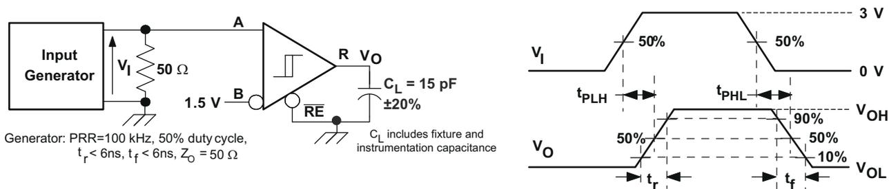
Figure 7-8. Receiver Switching Test Circuit and Waveforms
