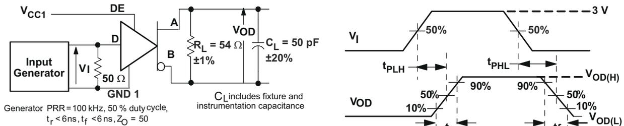
Figure 7-4. Driver Switching Test Circuit and Voltage Waveforms
