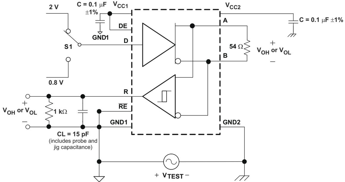
**Figure 7-12. Half-Duplex Common-Mode Transient Immunity Test Circuit**
