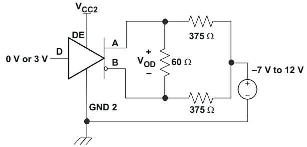
Figure 7-2. Driver  $V_{OD}$  With Common-Mode Loading Test Circuit
