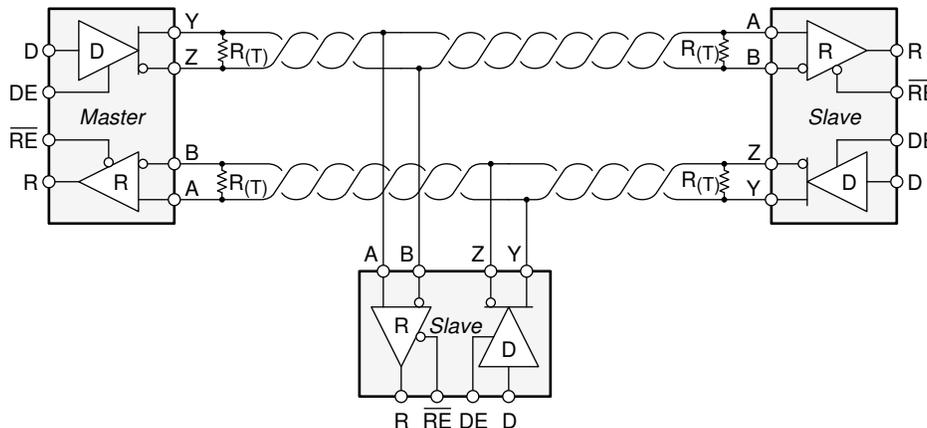
**Figure 9-2. Typical RS-485 Network With Full-Duplex Transceivers**
