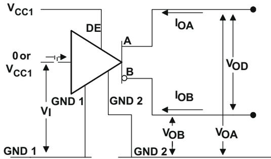
Figure 7-1. Driver  $V_{OD}$  Test and Current Definitions
