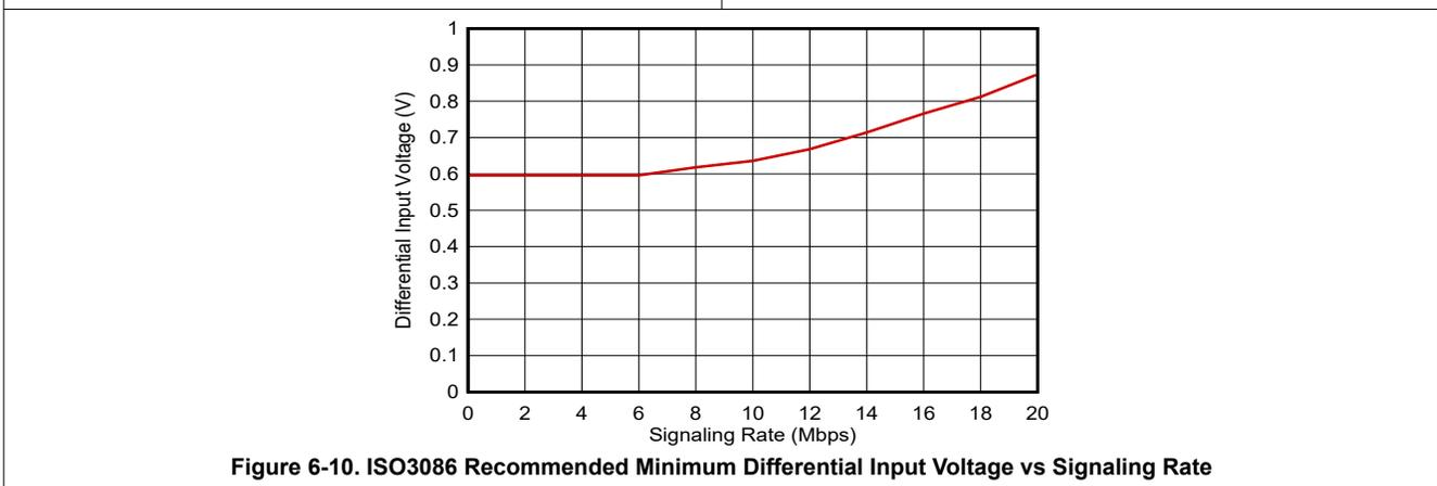
Figure 6-10. ISO3086 Recommended Minimum Differential Input Voltage vs Signaling Rate
