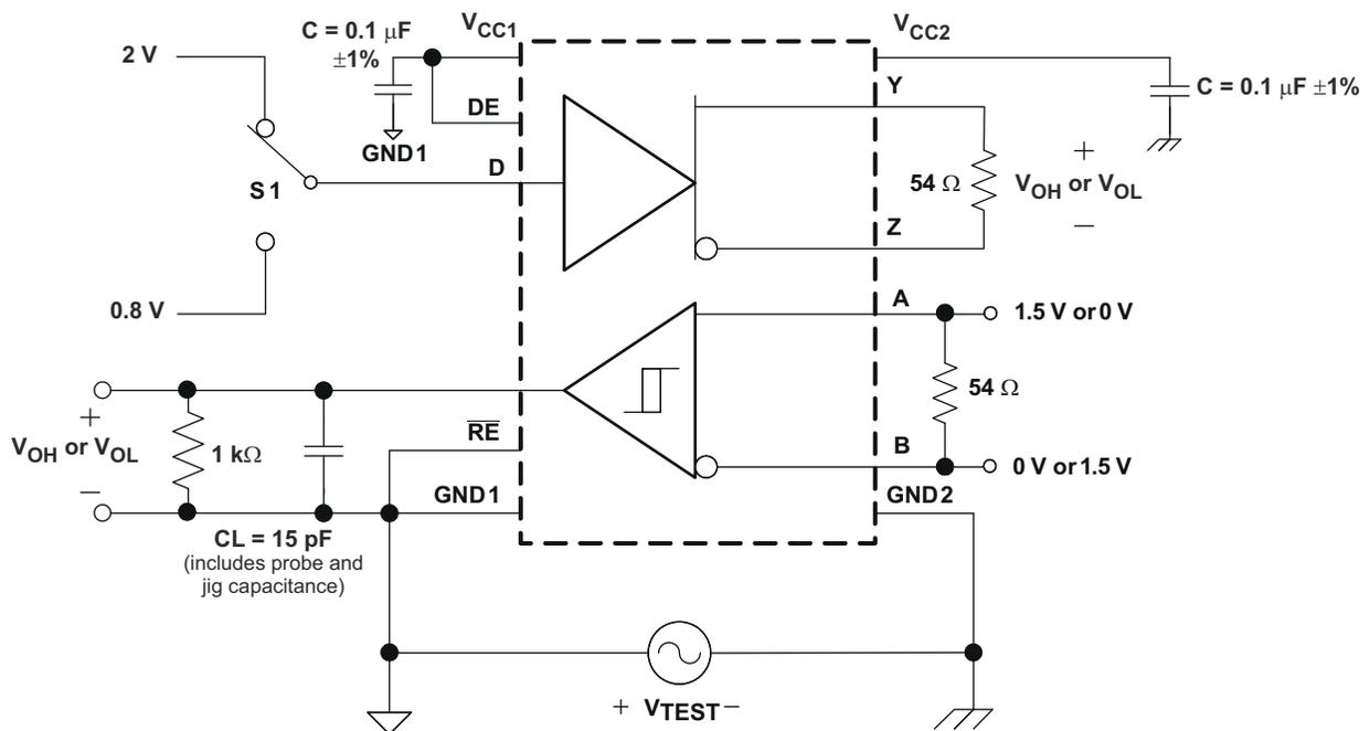
**Figure 7-13. Full-Duplex Common-Mode Transient Immunity Test Circuit**
