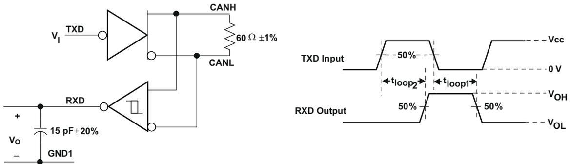
Figure 7-9.  $t_{LOOP}$  Test Circuit and Voltage Waveforms
