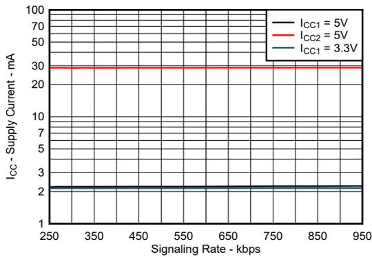
Figure 6-5. Supply Current (RMS) vs Signaling Rate (kbps)
