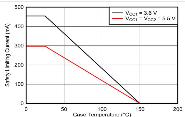
Figure 6-2. DW-16 Thermal Derating Curve per VDE
