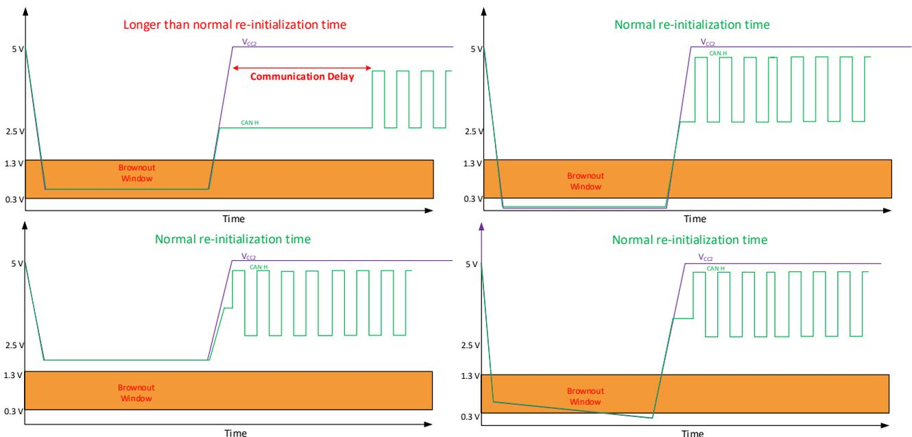
**Figure 10-1. Power Supply Ramp-Down and Communication Delay Behavior**
