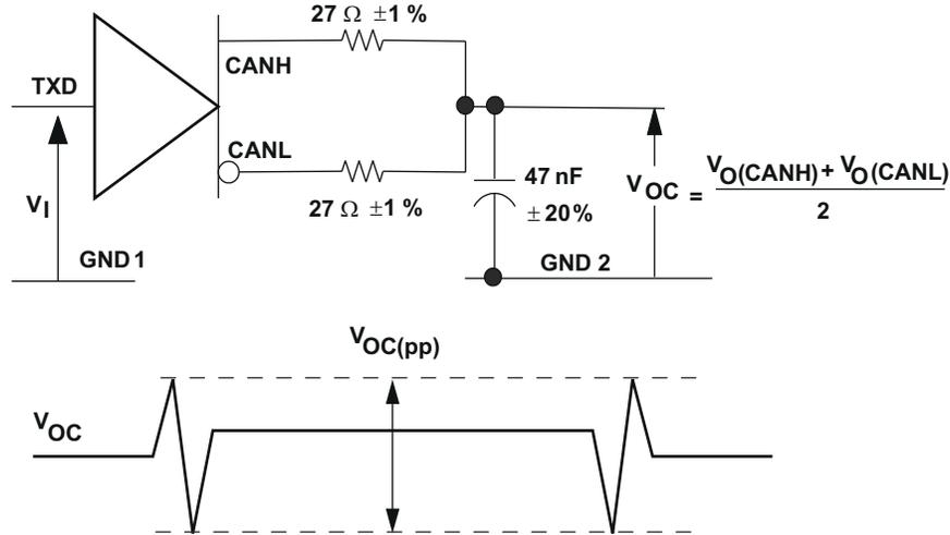
Figure 7-8. Peak-to-Peak Output Voltage Test Circuit and Waveform
