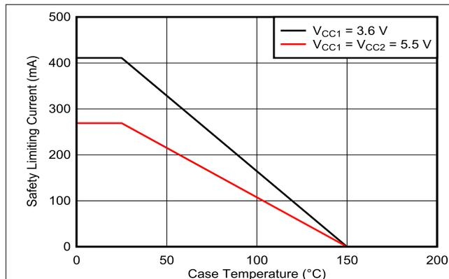
Figure 6-1. DUB-8 Thermal Derating Curve per VDE
