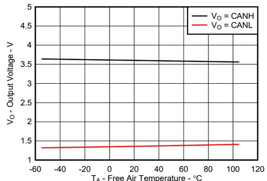
Figure 6-6. Driver Output Voltage vs Free-Air Temperature
