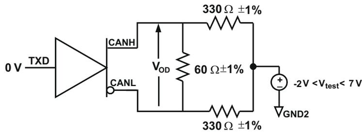
Figure 7-3. Driver  $V_{OD}$  With Common-Mode Loading Test Circuit
