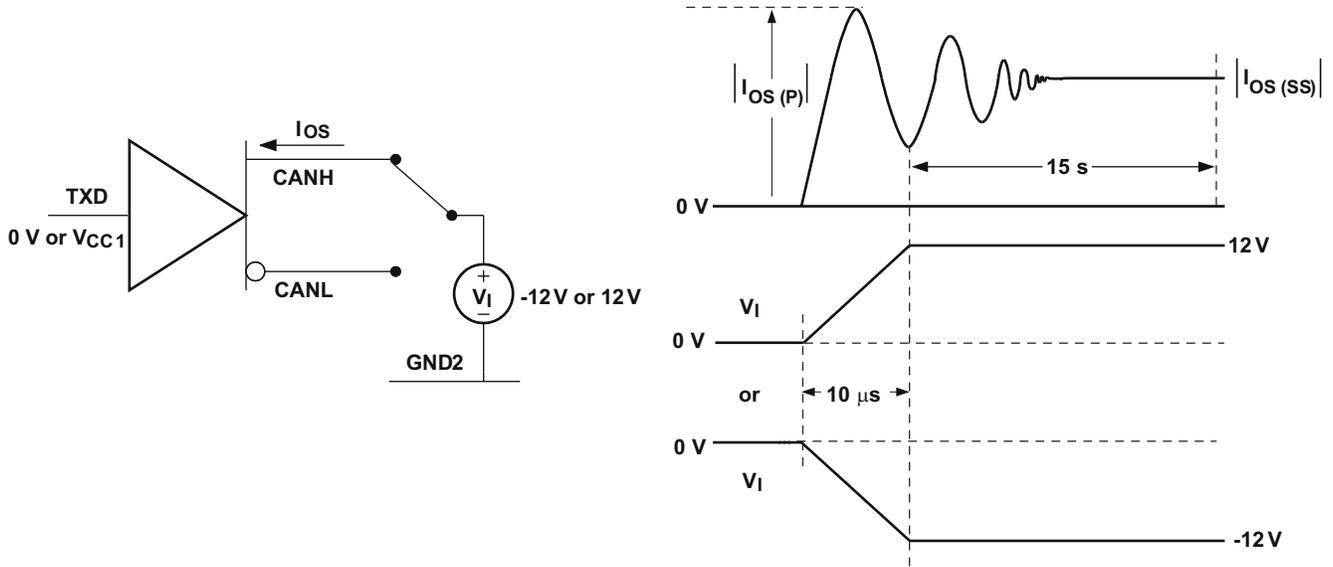
Figure 7-11. Driver Short-Circuit Current Test Circuit and Waveforms
