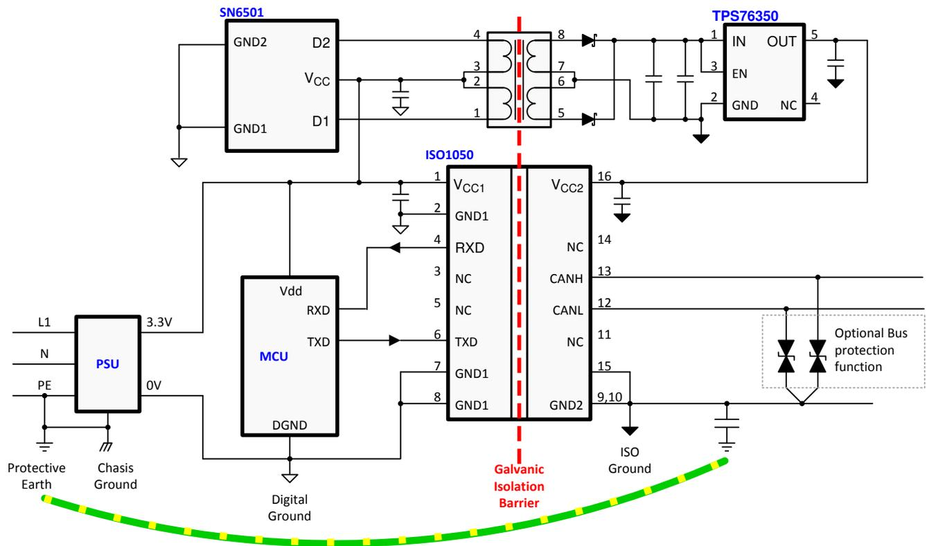
Figure 9-1. Application Circuit
